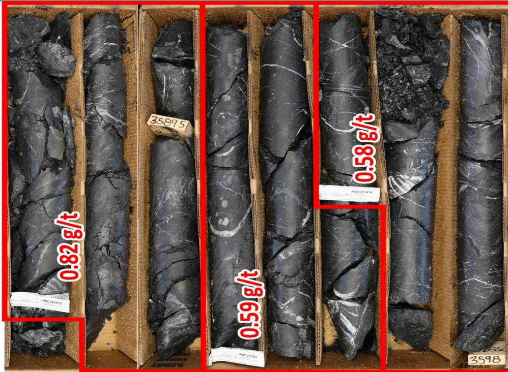
Figure 10-2: PW25-03 Lower plate showing carbonaceous laminated Wenban limestone
